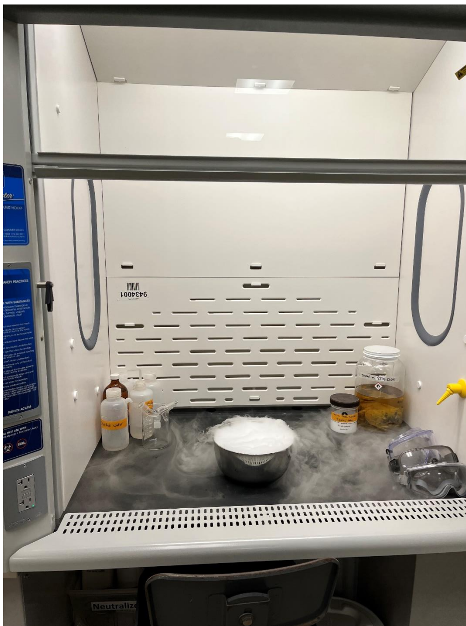
Figure 5: Sash all the way open (past stop) – Fumes are considered “lazy” and are not effectively exhausted. This is why the sash should never be opened past the sash stop during hazardous operations inside the fume hood.
