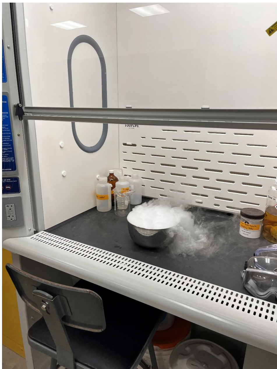
Figure 2: Sash opened to safe opening height (at sash stop) – Fumes are effectively exhausted.
