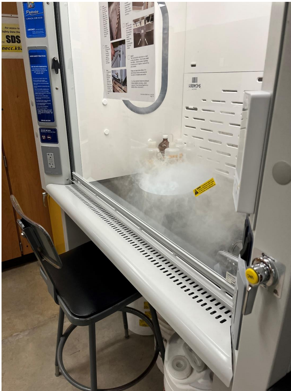
Figure 3: Sash Closed – Fumes are contained and effectively exhausted.
