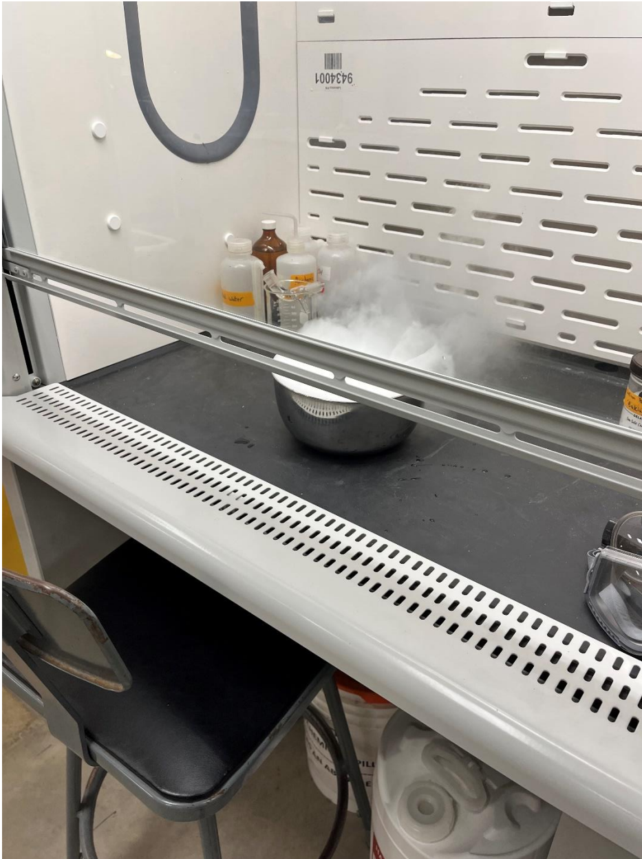
Figure 4: Sash slightly open – Fumes are effectively exhausted.
